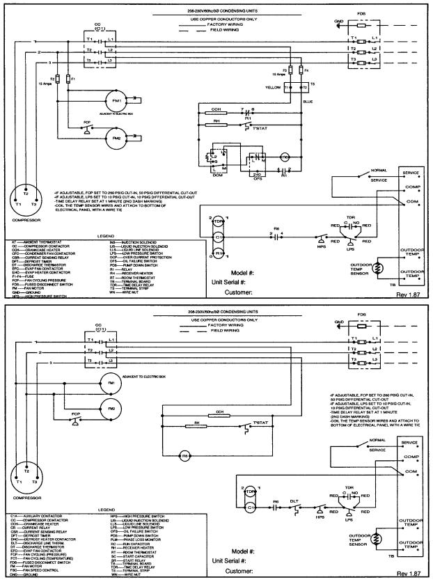
NOTE: THESE ARE TYPICAL CONDENSING UNIT WIRING DIAGRAMS. CONSULT WIRING DIAGRAM SHIPPED ON UNIT FOR ACTUAL UNIT WIRING.
