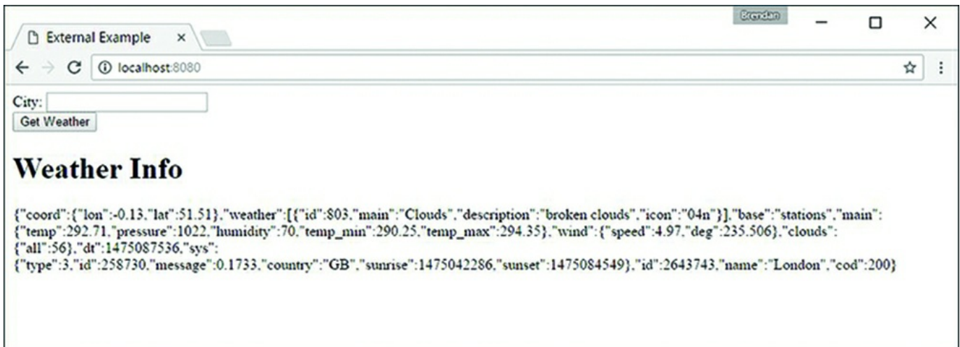
Figure 7.4 Implementing an external web service that connects to a remote source for weather data
