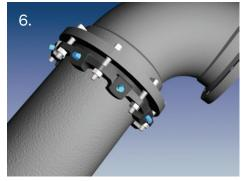
7. If removal is necessary, utilize the 5% inch hex heads provided. If reassembly is required, assemble the joint in the same manner as above, by tightening the wedge bolts to 90 ft-lbs. If the series 1100 restraint is removed from the pipe, be sure that all the collar bolts and wedges are in place before the restraint is reassembled.
