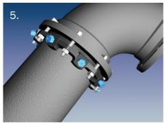
6. Tighten the torque limiting twist off nuts in a clockwise direction (direction indicated by arrow on top of nut) until all wedges are in firm contact with the pipe surface. Continue tightening in an alternating manner until all of the nuts have been twisted off.
