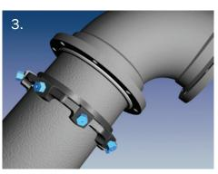
the requirement of ANSI/AWWA C111/A21.11, just prior to slipping the gasket onto the plain end for joint assembly. Place the gland on the plain end with lip extension toward the plain end, followed by the gasket.
