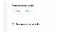
If the frame counter is checked, you must respect the sequence number, and probably copied packages are refused on the network. Though restarting you node, and thereby resetting the frame counter, will disable your node. So to get this working, you have to disable this check by unchecking this box. You can integrate the code of the bmp280 in the abp example.
