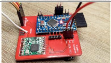
Put the Jumper on the FTDI board on 3.3V position!
