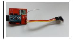
Connect the BME280 sensor with female-female jumper wires to the I2C connector: GND-> GND, SDA->SDA, SCL->SCL, VCC->+3.3V. The CSB en SDO are left open (only used in SPI connection). You can not connect straight forward, but you should twist the two wires in the middle.
