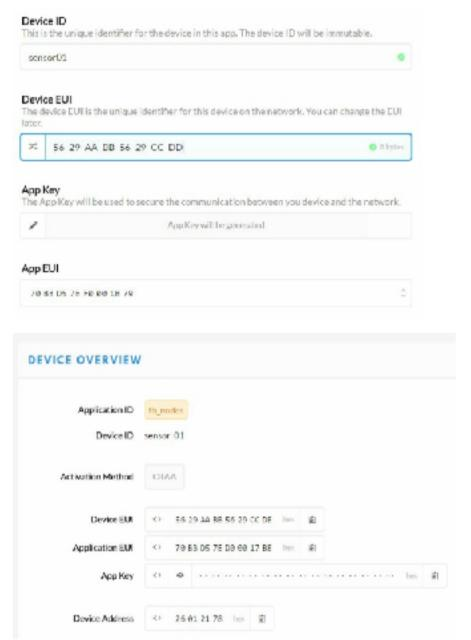
There are three values you should copy into your Arduino Code. Dev EUI (the device identifier), App EUI (The application identifier) and the App key.
