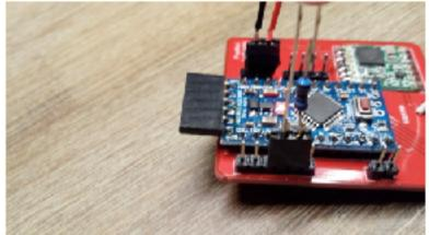
You can solder the battery holder on the pins GND (black) and 3.3V (red), you may use a female header here as well
