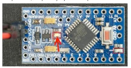
When you found the power LED, then try to locate at least one trace that leads to the LED. In the
