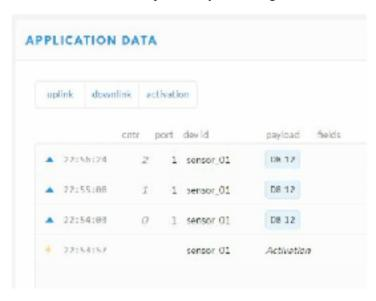
After a few minutes, the LED will stop blinking. You will see the information coming in into the dashboard. This is coded information, because some algorithm is used to put temperature and humidity in two bytes.
