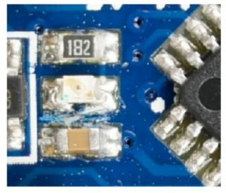
Removing the LEDs can be tricky, so it's easier to remove the series resistors for the LEDs instead. This version of Pro Mini also has a resistor feedback network for the regulator across VCC, these consume power so should be removed. Just push the resistors aside with a soldering iron. The picture shows the Pro Mini with unwanted parts removed, locations of the removed components are circled in red.
