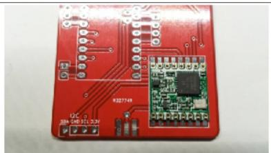
Align the solder pads and if the module is in place, solder the other pads. Do use as little as possible solder! Check the connections carefully!
