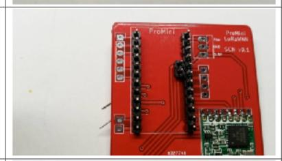
First solder the end pins, align the headers straight and solder all the other pins.
