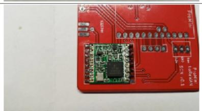
Put two 12p headers into the ProMini socket. Also put the 2p header inside the ProMini area. By holding them with a piece of paper you can turn around the PCB. (You can also use the ProMini to keep the pins in place by using an elastic band.)
