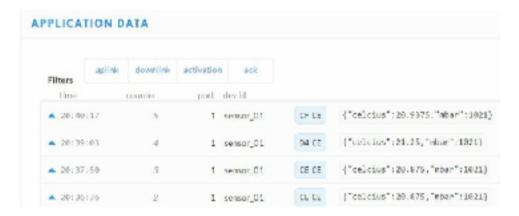
This way you can put several values into a byte string. Sending in clear ASCII is possible but due to bandwidth limitations not preferable in production environments. To make this even more scalable take a look at <a href="https://github.com/thesolarnomad/lora-serialization">https://github.com/thesolarnomad/lora-serialization</a>.
