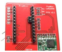
First solder the end pins, align the headers straight and solder all the other pins.
