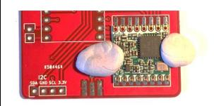
Align the solder pads and if the module is in place, solder the other pads. Do use as little as possible solder! Check the connections carefully!
