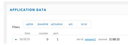
Note that the payload value is the same as the one that was printed by the Arduino program. This means that our data has made it through the connection. This is coded information, because the Arduino contains an algorithm that puts temperature, pressure and humidity into three bytes. This is
