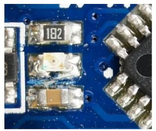
Removing the LEDs can be tricky, so it's easier to remove the series resistors for the LEDs instead. This version of Pro Mini also has a resistor feedback network for the regulator across VCC, these consume power so should be removed. Just push the resistors aside with a soldering iron. The picture shows the Pro Mini with unwanted parts removed, locations of the removed components are circled in red.
