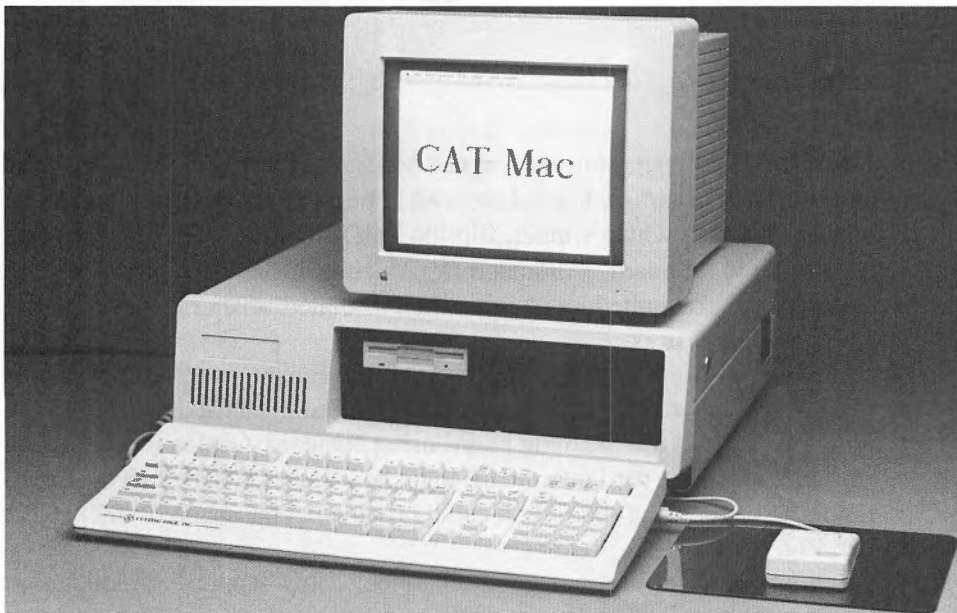
11-2 My first Cat Mac SE with an Apple monochrome monitor, Cutting Edge ADB Keyboard, and A+ ADB Optical Mouse.
