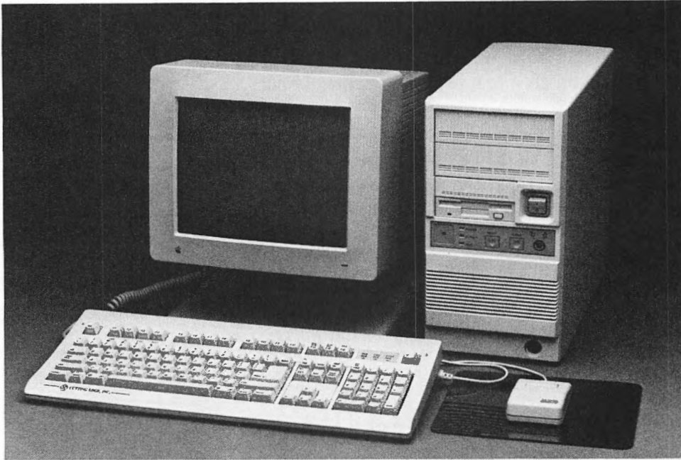
10-1 Cat Mac in mini tower PC case with Apple monochrome monitor on Ergotron tilt/swivel stand.
