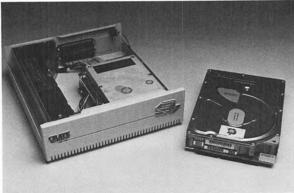
6-5 Close up of Wetex removable hard disk pak installed in low-profile Cat Mac case with drive pak partially removed.
