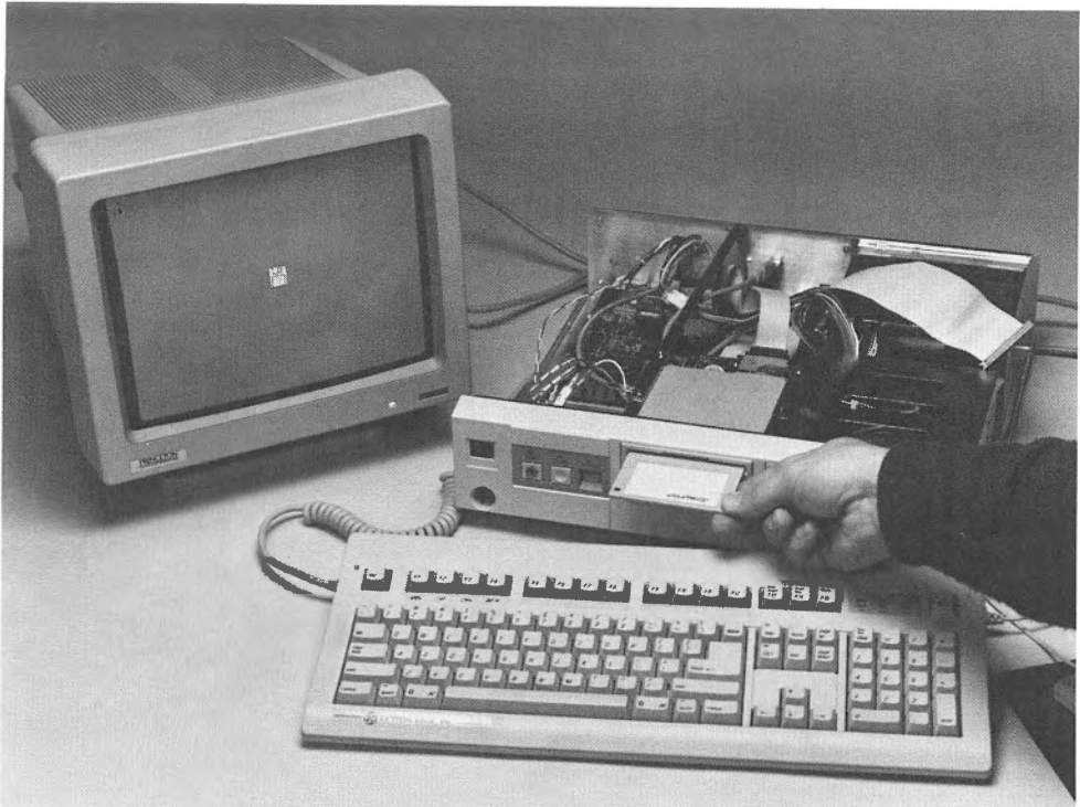
11-27 Loading the "Startup" disk. Notice question mark icon on screen and disconnected SCSI cable on top of disk drive bay.
