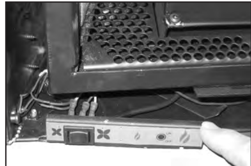
Figure 52. Remove/Install Control Panel.
