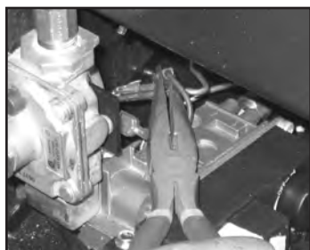
Figure 32: Remove Jumper From Thermocouple.
