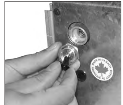
Figure 26: Set Gas Type for Valve.
