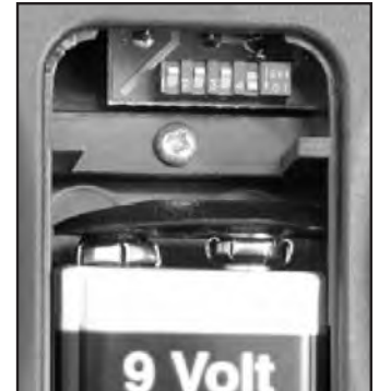
Figure 13: DIP Switch in Remote Handset Battery Compartment.
