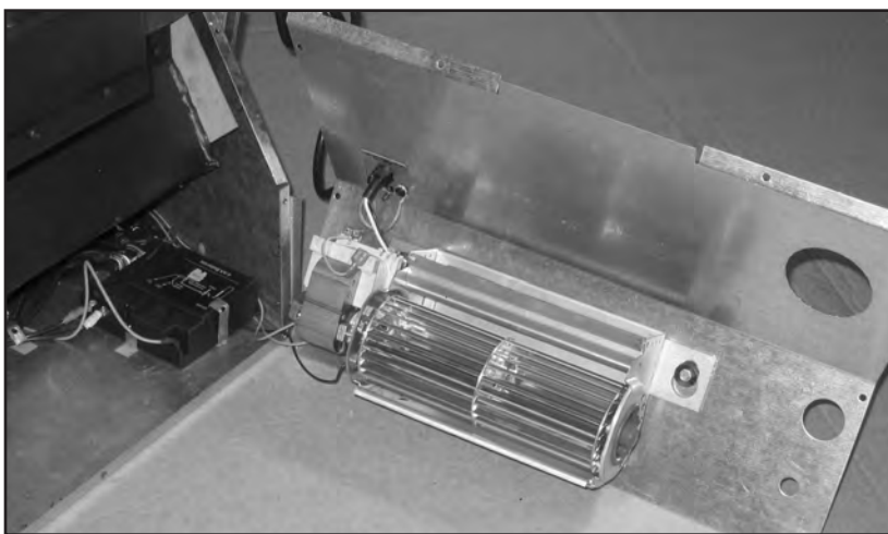
Figure 47: Installing Fan onto Back Panel.
