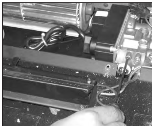
Figure 52: Opening Inlet Pressure Tap on Valve.
