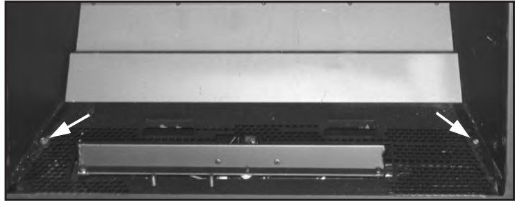
Figure 17: Screws Holding Burner Tray in Place.
