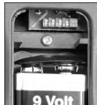
Figure 13: DIP Switch in Remote Handset Battery Compartment.
