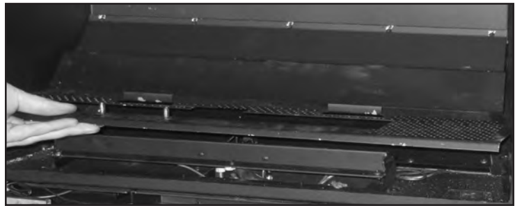
Figure 18: Removing Burner Tray.
