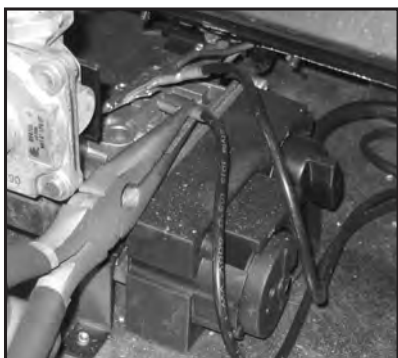
Figure 34: Remove Jumper From Thermocouple.
