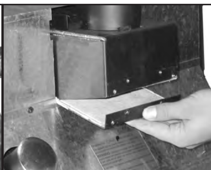
Figure 36: Remove Flue Slider Plate & Gasket.
