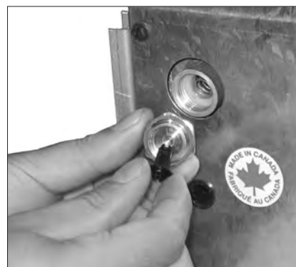
Figure 28: Set Gas Type for Valve.
