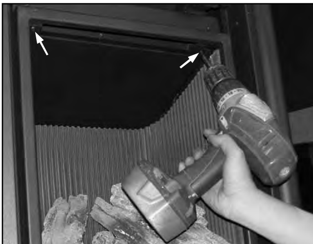
Figure 12: Firebox Baffle Screws Removal.
