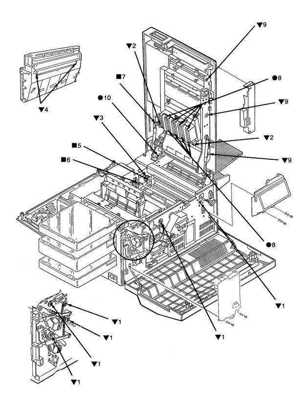
Figure 9-2. Front View Lubrication Points
