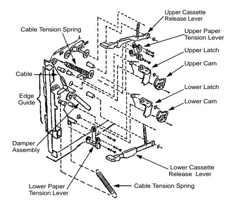
**14** Disengage the top of the damper assembly. Push it to the right out of the way.
