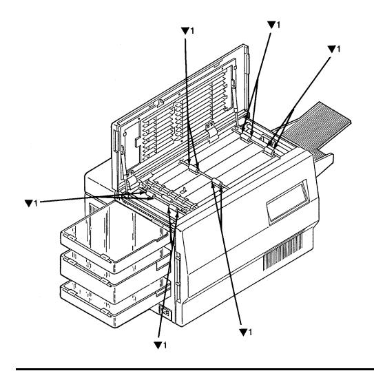
Figure 9-4. Duplex Only: Top View Lubrication
