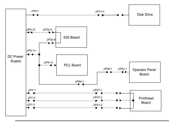
Figure 6-2. (Simplex) +5 Vdc Circuit
