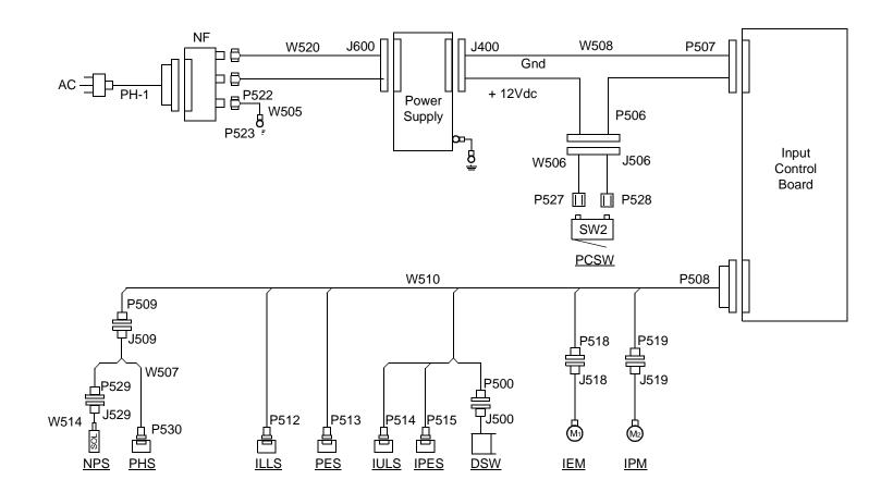
Figure 8-3. Connection Diagram for 1200-Sheet/2500-Sheet Feeder
