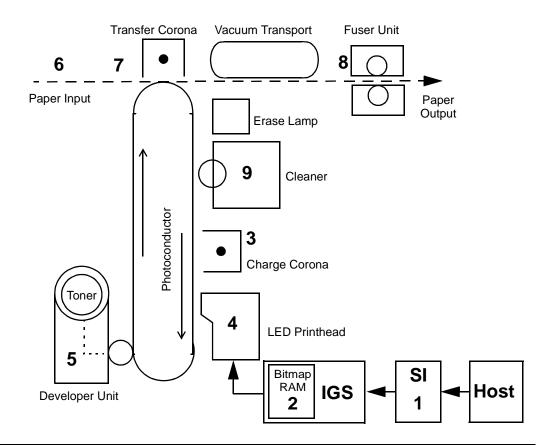
Figure 1-1. Cycle of Operation
