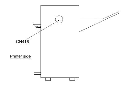
Figure 8-6. Connector Locations (front view, cover removed)
