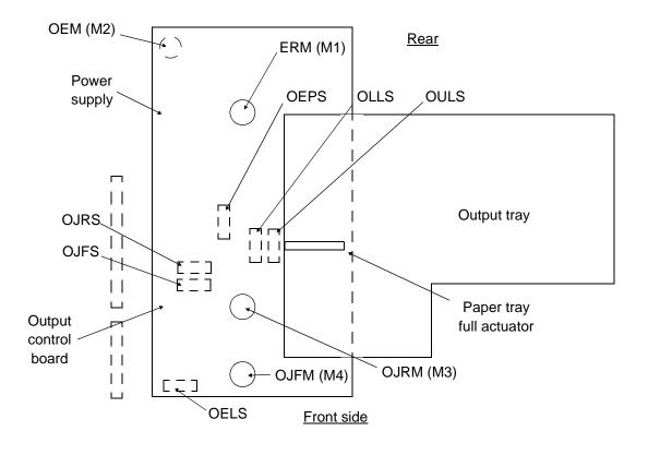
Figure 8-4. 1400-Sheet Stacker Component Locations
