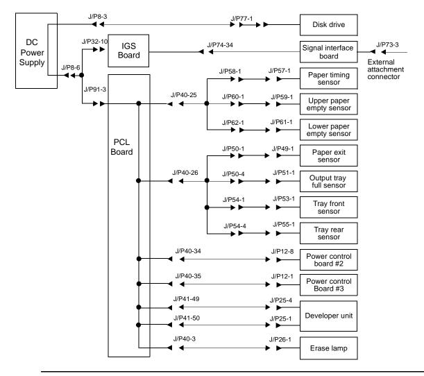
Figure 6-3. (Simplex) +12 Vdc Circuits
