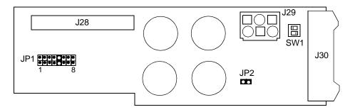
Figure 6-11. Printhead Circuit Board Jumper/Switch Locations
