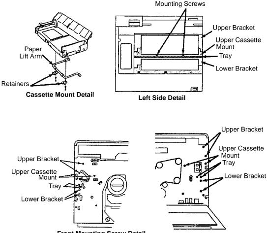
Front Mounting Screw Detail Back Mounting Screw Detail
