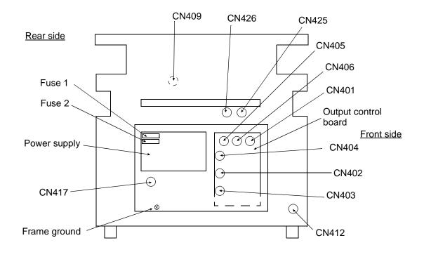
Figure 8-7. Connector Locations (left side view, left cover removed)
