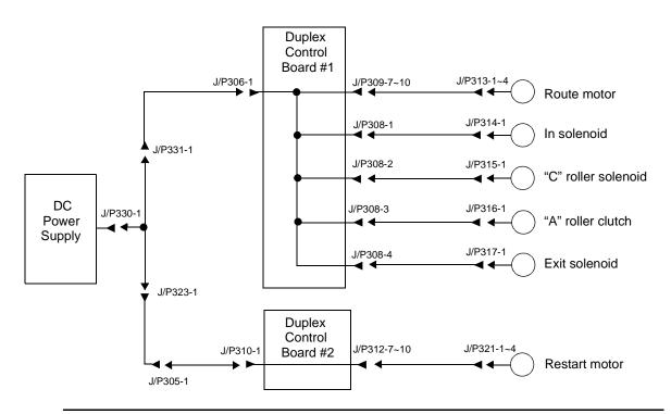
Figure 6-6. (Duplex) +24 Vdc Circuits
