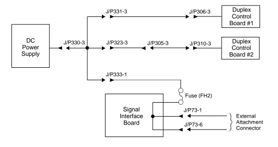
Figure 6-5. (Duplex) +5 Vdc Circuit
