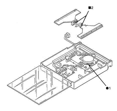
Figure 9-5. Duplex Only: Duplex Holding Tray Lubrication
