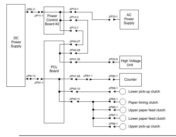
Figure 6-4. (Simplex) +24 Vdc Circuits
