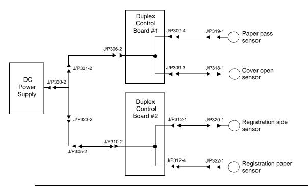
Figure 6-7. (Duplex) +12 Vdc Circuits
