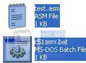
Figure 2-8. Assembling a file by drag and drop on top of batch file
