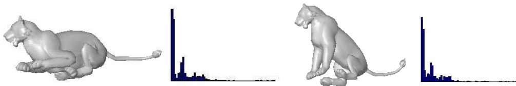
Fig. 2: Similar signatures are obtained based on the cross-sections for pose invariant lion models.
