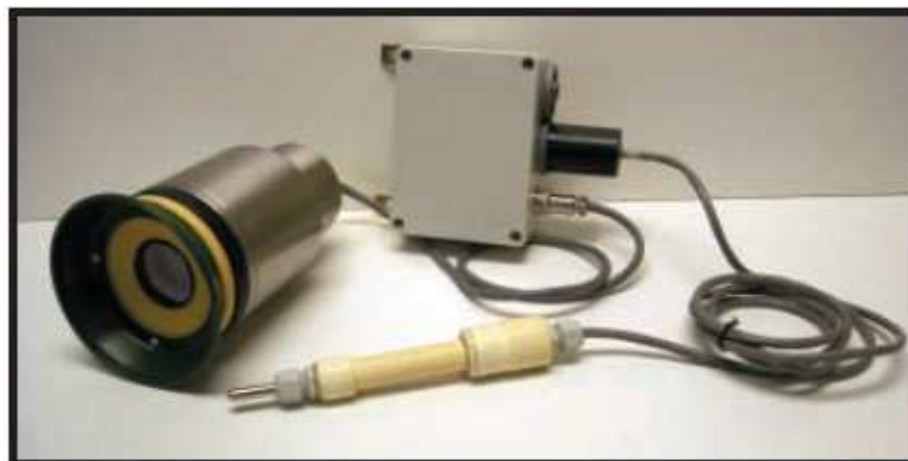
Photo 2—The snow depth sensor's electronic parts are ready for installation on the mounting structure. The temperature sensor will be mounted in a solar radiation shield to prevent excessive heating. The plastic film cans protect the connectors from the elements.
