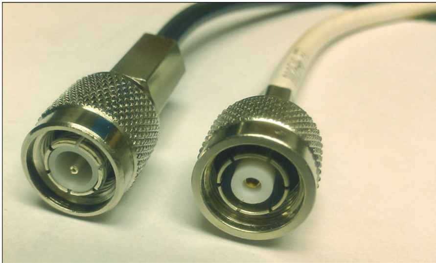
Figure 2-1 A Comparison Between TNC (left) and Cisco RP-TNC Connector (right).
