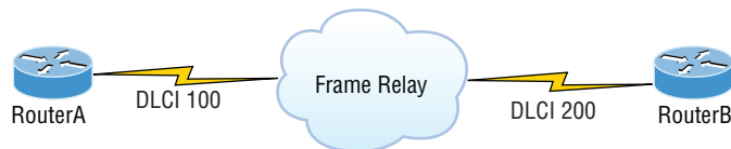
FIGURE 21.20 Frame Relay mappings
