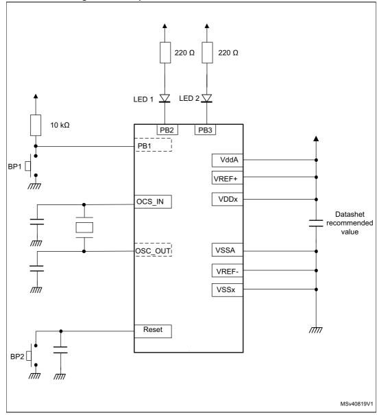
Figure 7. Example of test board schematics for STM32
