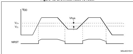
Figure 12. Brownout reset vs reset
