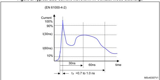
Figure 2. Typical ESD current waveform in Contact-mode discharge
