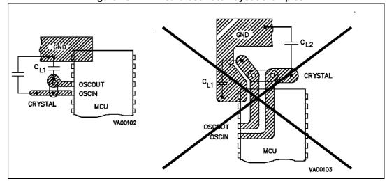
Figure 18. PCB Board oscillator layout examples
