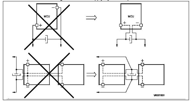
Figure 20. Power supply layout examples
