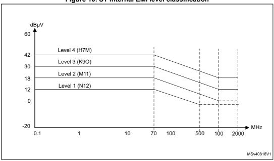
Note: To comply with level 2: no peak detection above 1 GHz.
