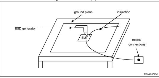
Figure 1. ESD test equipment
