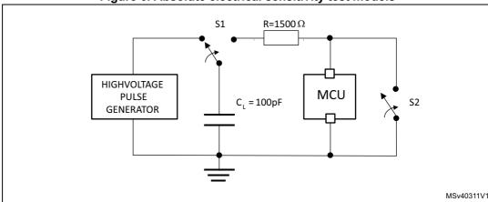
Figure 6. Absolute electrical sensitivity test models
