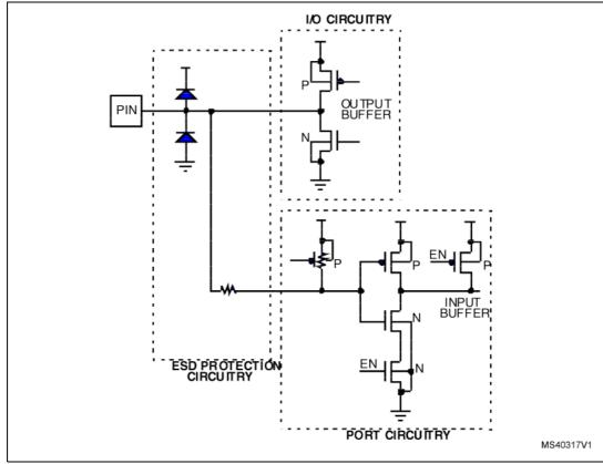
Figure 14. Digital input/output - push-pull
