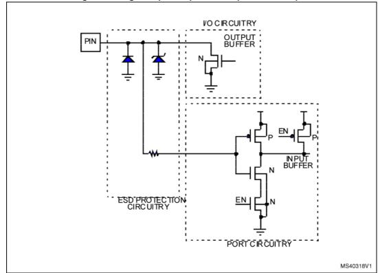
Figure 15. Digital input/output - true open drain output
