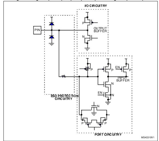
Figure 16. Digital input/output - push-pull output - analog multiplexer input
