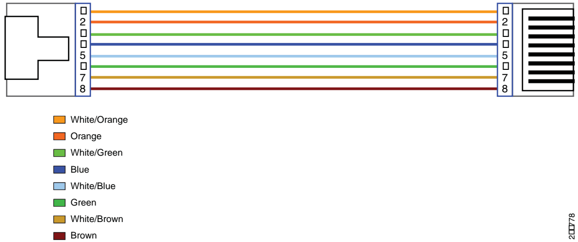
Figure B-5 Pin Assignments and Wiring for an RJ-45 Crossover Cable
