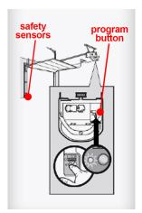
Your garage door opener must have safety reversing sensors which can be found at the bottom of the track of the door. These sensor prevent the door from closing when there is something blocking the path of the door.
