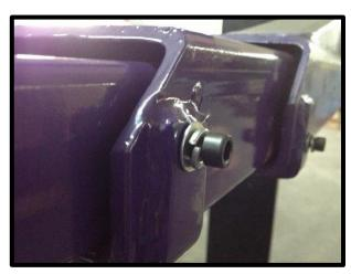
Install Arm Lock Latches W/Spring, Washer, and Retaining Pin On Bottom of Arm Adjust Arm Locks So The Teeth Interlock When The Lift Is Raised
