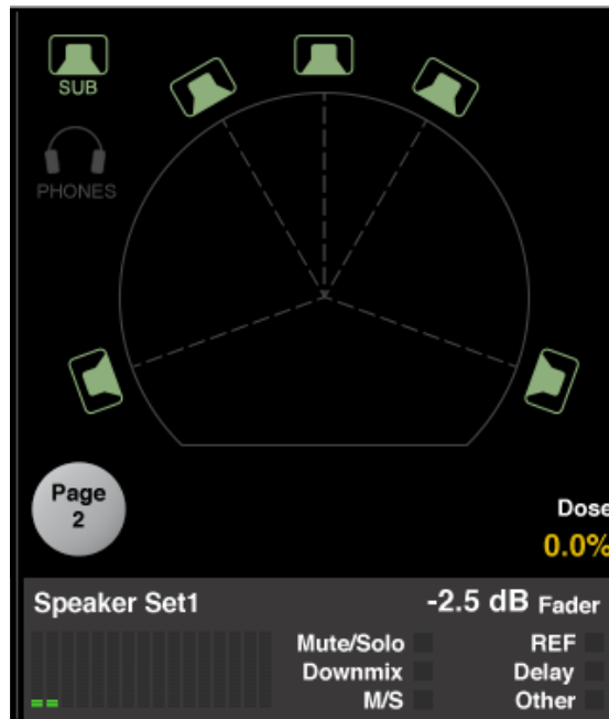
Fig. 65: Clarity X Main View, right pane, page 1 showing the current speaker set, the Dose Meter, the Speaker Set overview, and various status indicators
