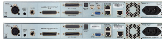
Fig. 10: Clarity X hardware options: With MADI (top) and without MADI (bottom)
