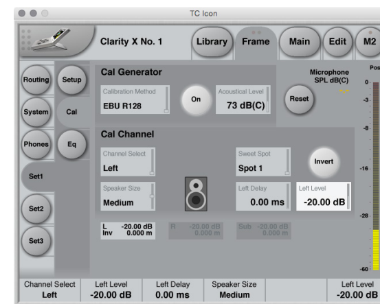
Fig. 49: Calibrating the left speaker in a 5.1 setup to EBU R128
