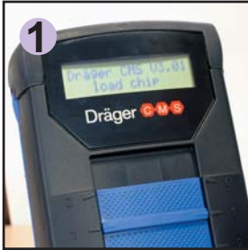
1 Turn on unit by moving the slide to position 1. Wait for "load chip" prompt.
