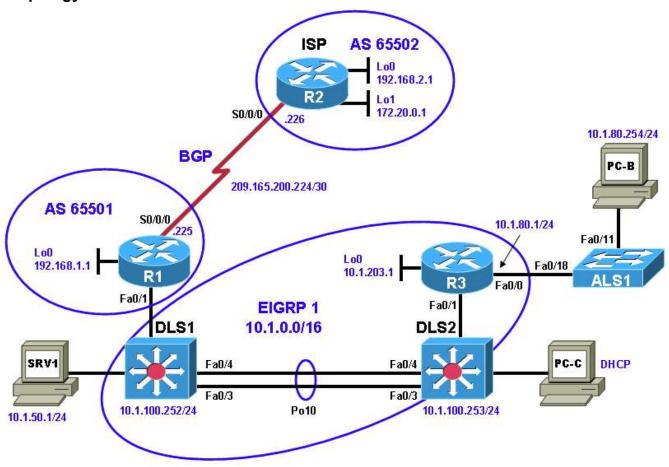
**Note:** The topology for this lab moves access switch ALS1 to R3 and disconnects it from switches DLS1 and DLS2. This allows a load to be placed on R3 using ALS1 and DLS2. PC-B is moved to switch ALS1 port Fa0/11. Performance testing is done using Cisco IOS commands on R3 and pings from PC-B. Even though ALS1 is no longer attached to DSL1 and DLS2, VLAN 10 still exists. The interfaces for port channel 1 on DLS1 and port channel 2 on DLS2 are temporarily shutdown.
