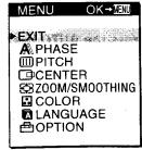
The OSD automatically disappears after about 30 seconds. To close the OSD, press the MENU button again.
