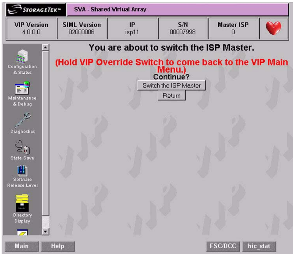
Figure 48 Switch ISP Master Screen
