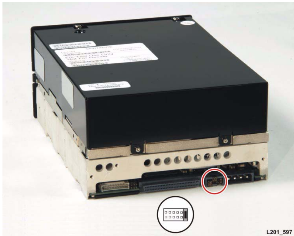
Figure 4-19. Quantum Certance Drive Terminating Power Jumpers
