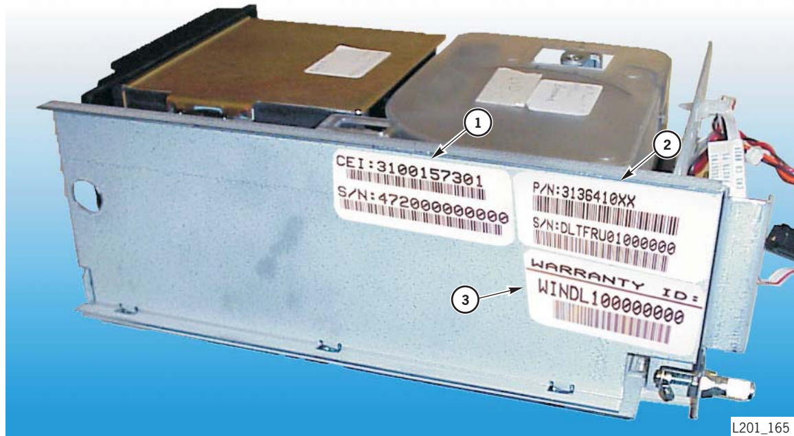
Figure 1-7. Ultrium LTO Drive Serial Number, Warranty Identification Number Locations (L201_165)
