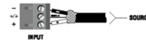
Figure 3.3 Balanced Input Connector Wiring
