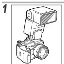
Attach the flash to the camera's hot shoe.
