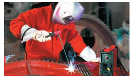
Rebuilding gear teeth
