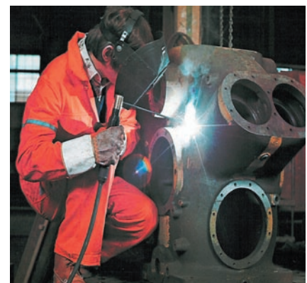
The ability to "cold" weld cast iron "in-position" with Xuper 2240 facilitates repair of big, complex, costly castings.
