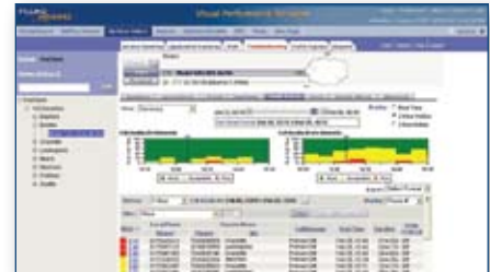
See application traffic traversing the router broken down into specific applications and their capacity usage.
