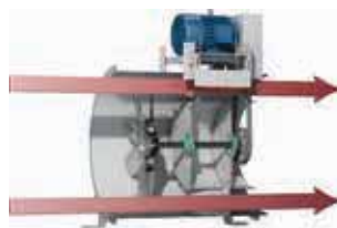
Axial Fan: Straight-through, nearly linear airflow.
