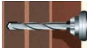
① Drill hole with percussion drill
