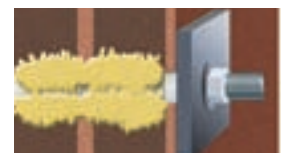
⑨ Install component, apply torque
