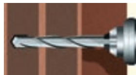
① Drill hole with percussion drill
