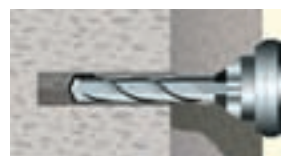
① Drill hole with percussion drill
