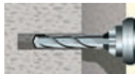
① Drill hole with percussion drill
