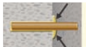
⑦ Visual check of mortar filling
