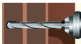
① Drill hole with percussion drill
