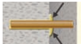
⑦ Visual check of mortar filling
