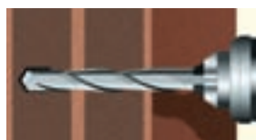
① Drill hole with percussion drill
