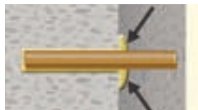
⑦ Visual check of mortar filling
