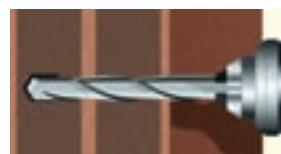
① Drill hole with percussion drill
