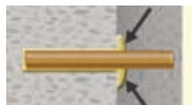
⑦ Visual check of mortar filling
