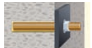
⑨ Install component, apply torque
