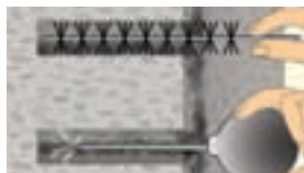
② Clean drill hole (blow out: 4x, brush out: 4x, blow out: 4x)
