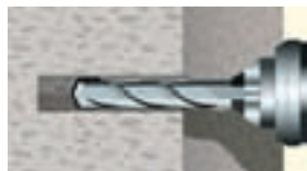
① Drill hole with percussion drill
