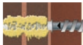
⑦ Push anchor into base of sleeve while turning clockwise
