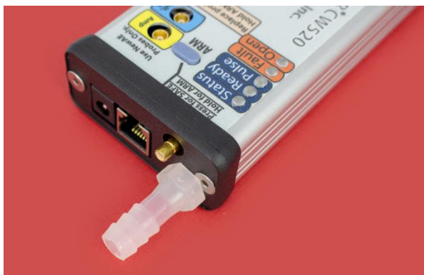
Figure 12: Adding air inlet adapter.
