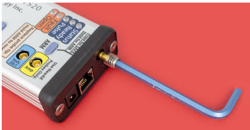
Figure 11: Removing blanking plug.
