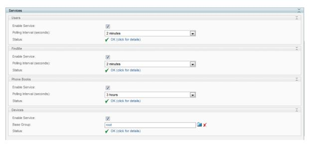
8. When green check marks are displayed for all services, scroll to the **VCS Provisioning Mode** field at the top of the page and select *Provisioning Extension*. Click **Save**.
