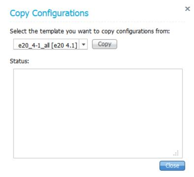
ii. Select the template from which you want to copy all configurations, and then click Copy. The Status field reports the result of the copy. The number of successfully copied configurations is displayed, as well as the number that failed to copy, for example, due to the target template's schema not supporting the same keys as the originating template's schema.
