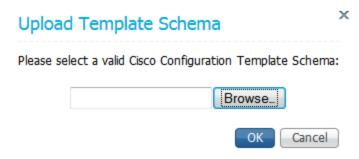
4. Click the **Browse** button, navigate to the folder on your local server to where you downloaded the schema, select it, and then click **OK**. The template schema is added in the relevant folder for the relevant model and version of device.
