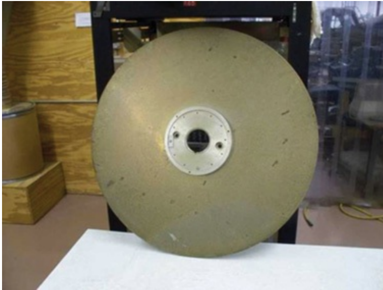
Figure A.3 One platter of that disk: 3/8 inch thick, 36 inches in diameter
