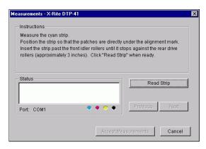
Align the page in the measurement page slot of the DTP41 so that the appropriate color column is centered below the alignment mark. Insert the page about three inches, past the front idler rollers, until it rests against the rear drive rollers and you feel resistance.
