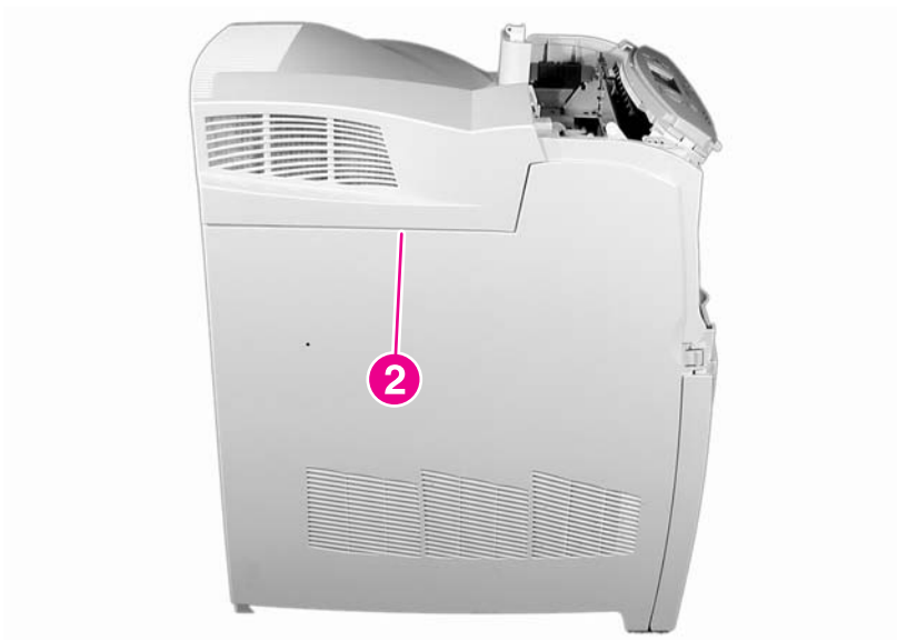
Figure 6-7 Remove the rear top cover (3 of 3)
