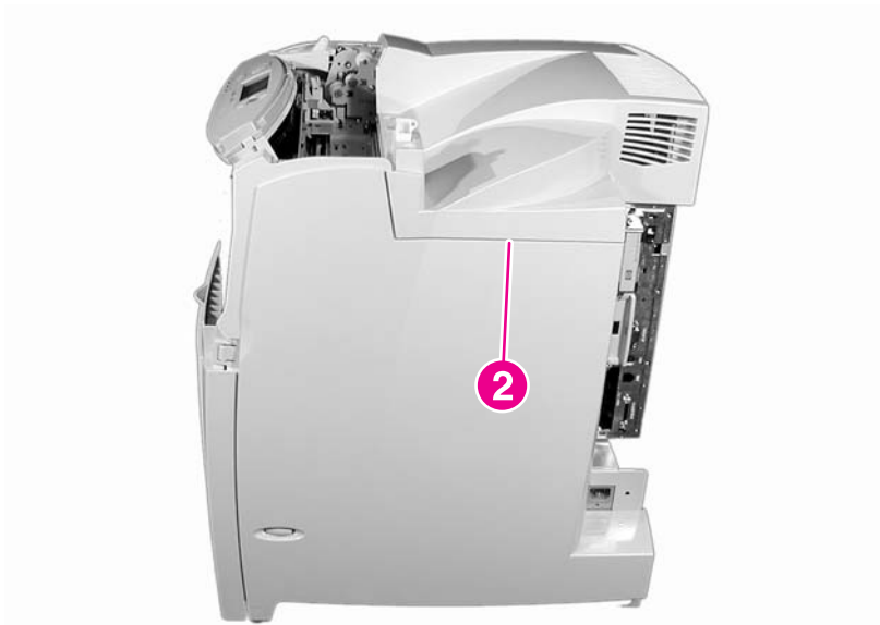
Figure 6-6 Remove the rear top cover (2 of 3)
