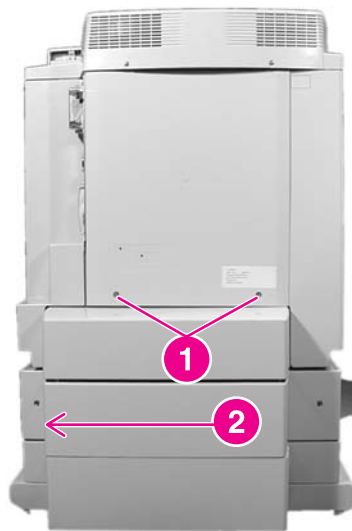
Figure 6-3. Removing and replacing the rear cover
