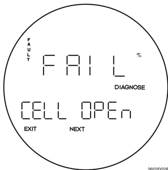
Figure 6-9. Fault 5, O 2 Cell Open
