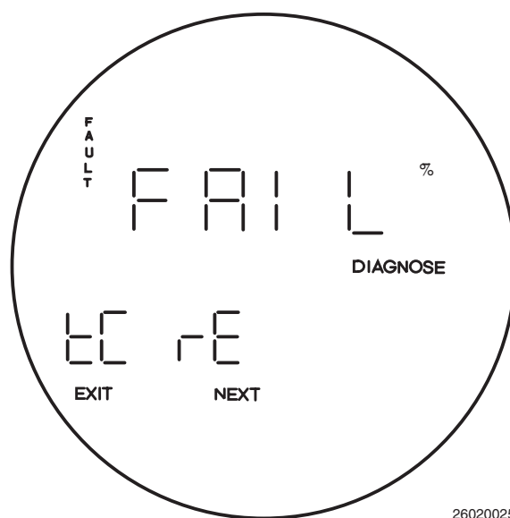
Figure 6-6. Fault 2, Reversed Thermocouple
