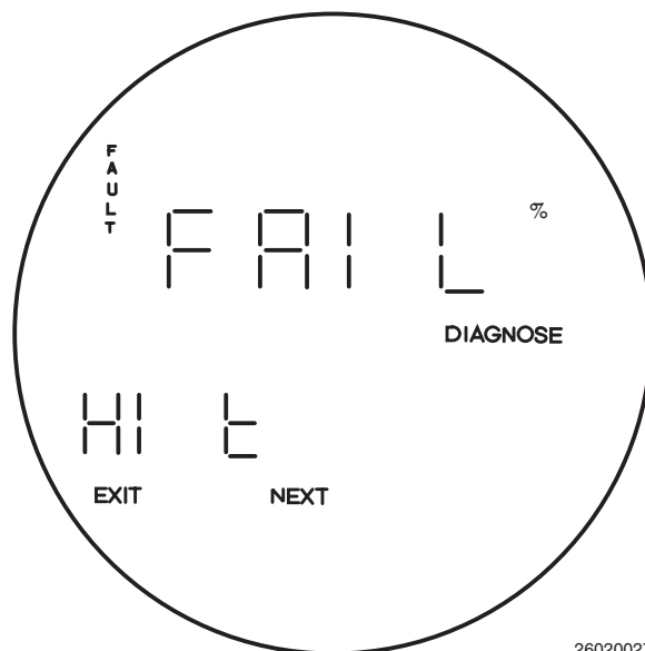
Figure 6-8. Fault 4, High Probe Temperature
