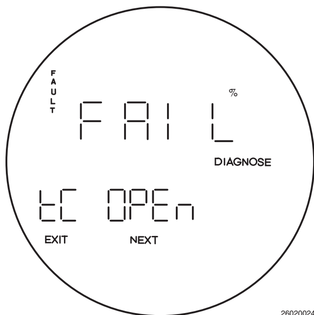
Figure 6-5. Fault 1, Open Thermocouple
