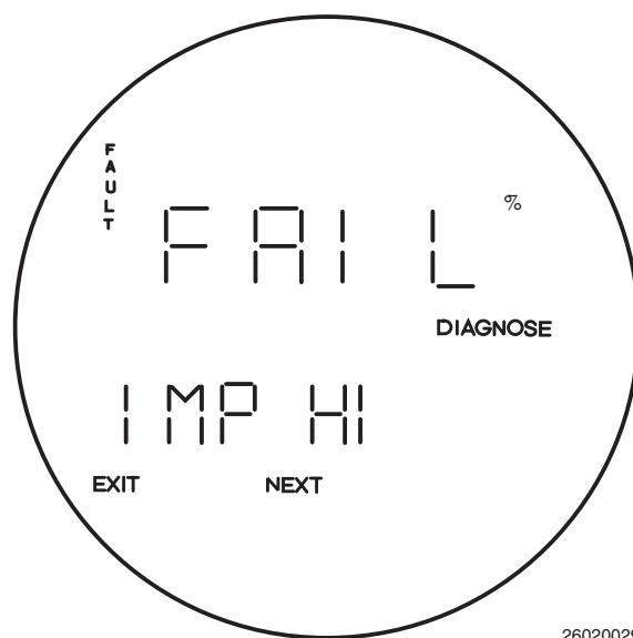
Figure 6-10. Fault 6, Cell Impedance Too High
