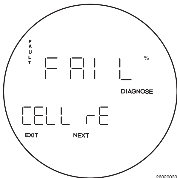
Figure 6-11. Fault 7, Reversed O 2 Cell
