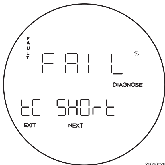
Figure 6-7. Fault 3, Shorted Thermocouple
