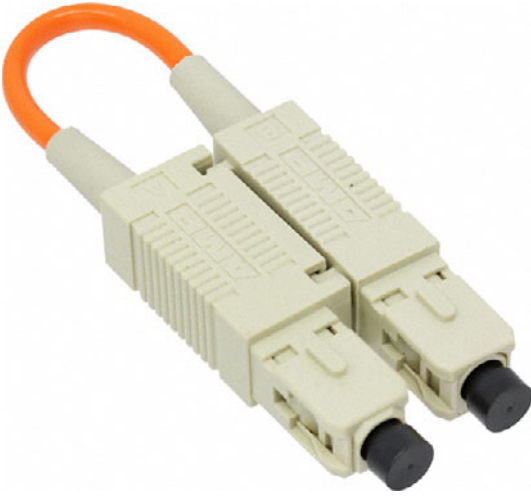
Figure 11-4 Fiber-Optic Loopback Plug (Photo Courtesy of Digi-Key Corporation [www.digikey.com])
