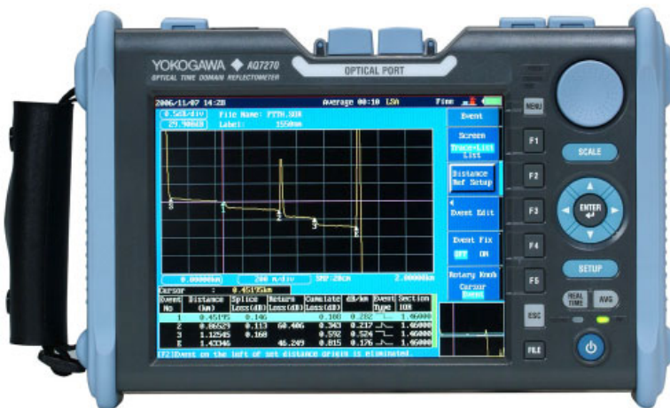
Figure 11-8 Optical Time Domain Reflectometer (Photo Courtesy of Coral-i Solutions [www.coral-i.com])
