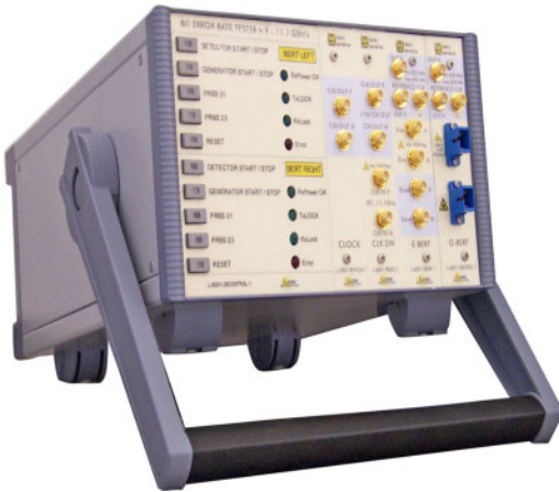
Figure 11-1 Bit-Error Rate Tester (BERT) (Photo Courtesy of BBN International [www.bbnint.co.uk])
