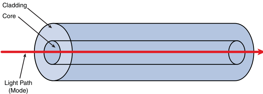
Figure 3-8 Light Propagation in Single-Mode Fiber
