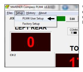
When you connect new load cells to the Compass PLM4, you need to set up the Compass PLM4 with proper parameters for each load cell connected in PLM4 User Setup screen.
