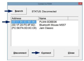
Note: Once the connection is made to the CompassPLM4, MarinerCP will try to connect to the same CompassPLM4 automatically every time the program starts. If you need to connect to different CompassPLM4 while connected the other already, from the top main menu, select Setup>Connect to PLM4 to bring up the search screen.
