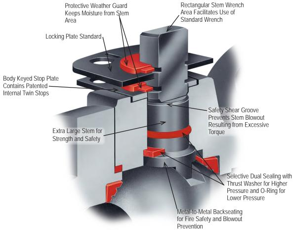
In keeping with Balon's philosophy of design which envisions simplification and improvement instead of improvement by complication, the Balon stem design solves many problems associated with the common stem design. The overall utility of the ball valve is related in no small way to the basic stem design. Certain standard designs originated early and were followed through by ball valve manufacturers in the years following the advent of the ball valve itself during World War II.
