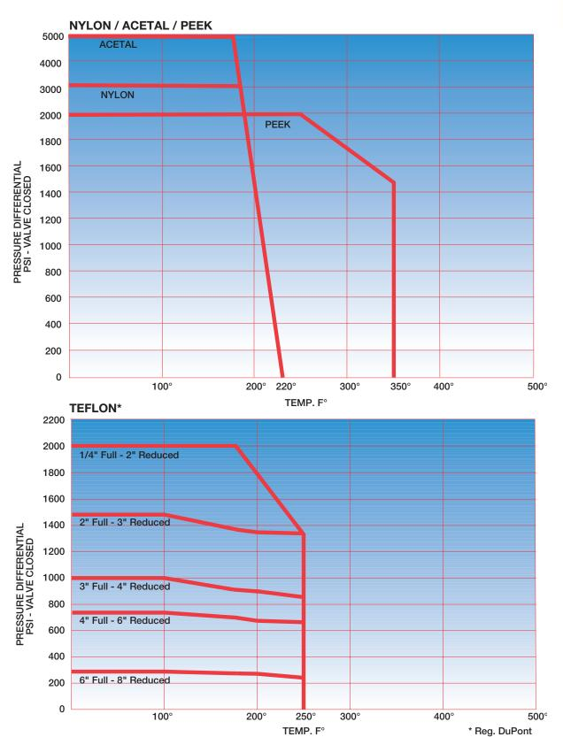
All Balon valves are rated for a minimum temperature of -20° F except for valves designated as low temperature valves, which are rated for a minimum temperature of -50° F.
