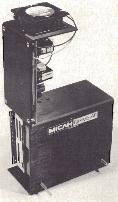
The MicahDrive AT internal hard disk drive for the Macintosh 512 and Macintosh Plus.
