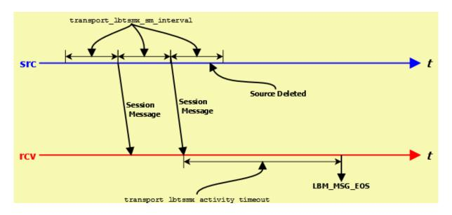
The Source Session Message mechanism enables the receiver to detect when a source goes away and works similarly to LBT-RU. It operates independently of message writes/reads in the Shared Memory Area.
