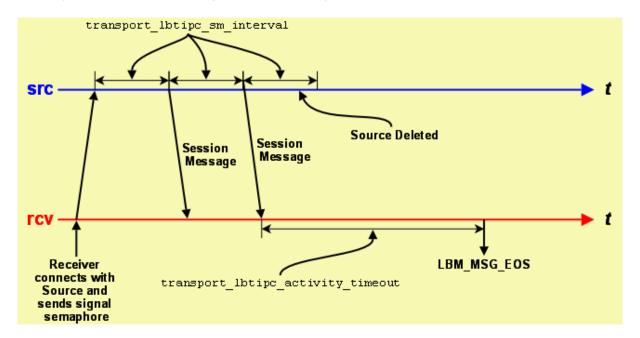
The Source Session Message mechanism enables the receiver to detect when a source goes away and works similarly to LBT-RU. It operates independently of message writes/reads in the Shared Memory Area.
