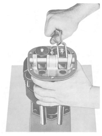
Figure 19. Compressing Valve Spring to Remove Locks
