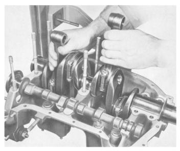
Figure 32. Installing Crankshaft and Connecting Rods.
