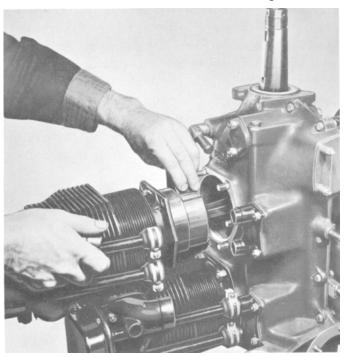
Figure 37. Installing No. 3 Cylinder.
