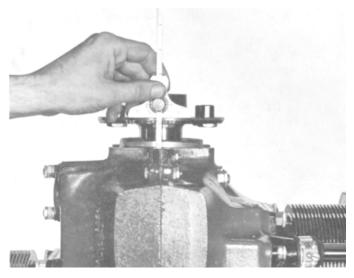
Figure 40. Placing Flange Crankshaft in Firing Position of No.1 Piston.
