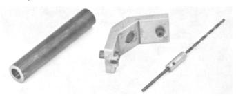
Figure 27. Drill Fixture.
