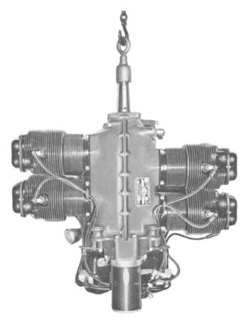
Figure 11. Hoisting Engine by Crankshaft Lifting Eye.
