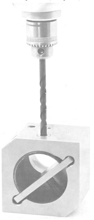
Figure 24. Drilling Hole in Bearing
