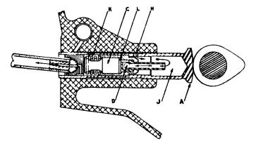
Figure 8. Section Through Hydraulic Valve Lifter.
