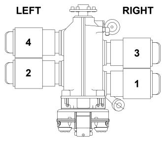
Figure 7. Cylinder Arrangement Diagram (Top View
