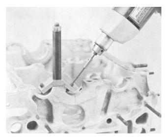
Figure 28. Drill Fixture Installed
