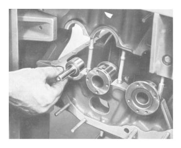
Installing Starter Pinion Pivot Manual Starting Engines.
