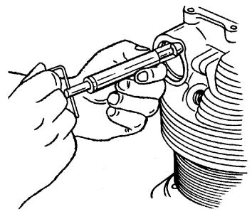
Figure 21. Installing Helical Coil Inserts
