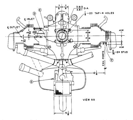
Figure 13. Installation Drawing for –12, -14 & -16 Models, Front View.
