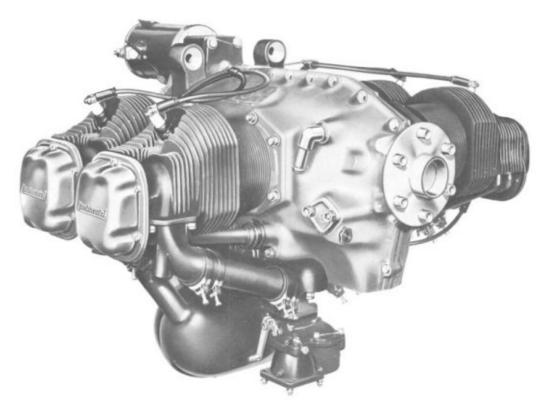
Figure 5. Right Front View, Model C90.
