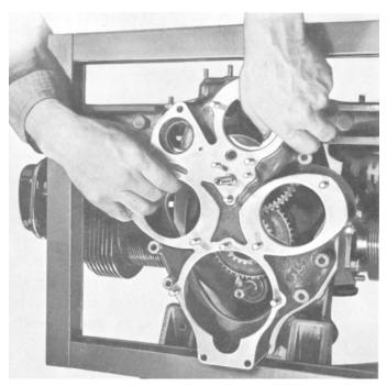
Figure 36. Installing Crankcase Cover on -12, -14, -16 and O-200 Models.
