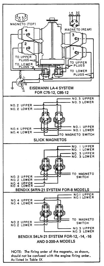
Figure 17. Ignition Wiring Diagram.
