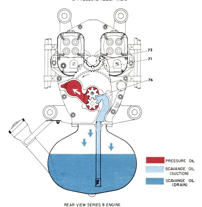
Figure 46. Limits and Lubrication Chart (Sheet 3 of 4) – Rear View and Horizontal Section, -8 Model.
