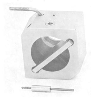
Figure 23. Drill Fixture
