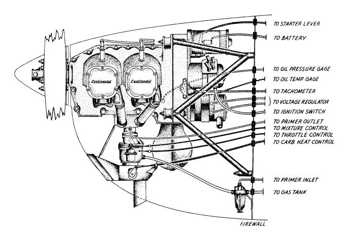
Figure 12. Typical Installation Diagram for -12, -14 & -16 Models, Side View.
