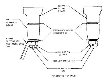
Figure 38. Install "O" Rings on Intake Manifold Studs.
