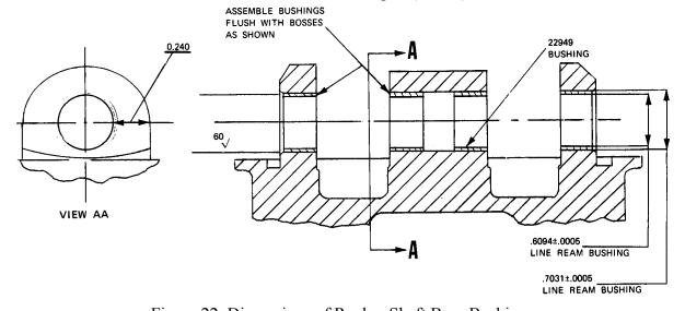
Figure 22. Dimensions of Rocker Shaft Boss Bushings
