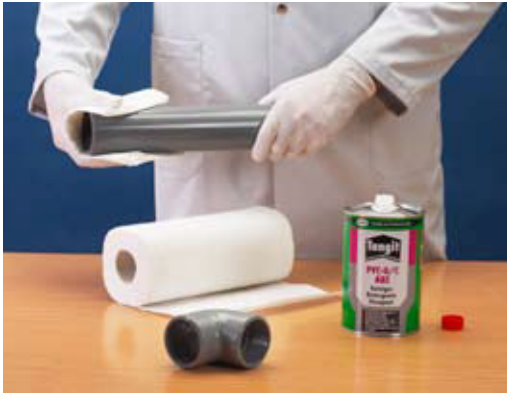
Cleaning the pipe and socket
