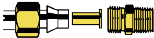
Plastic Sleeve / Insert Assembly
