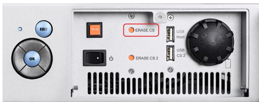
Figure 15: ERASE pushbutton for performing External Erase on a CryptoServer LAN V4
