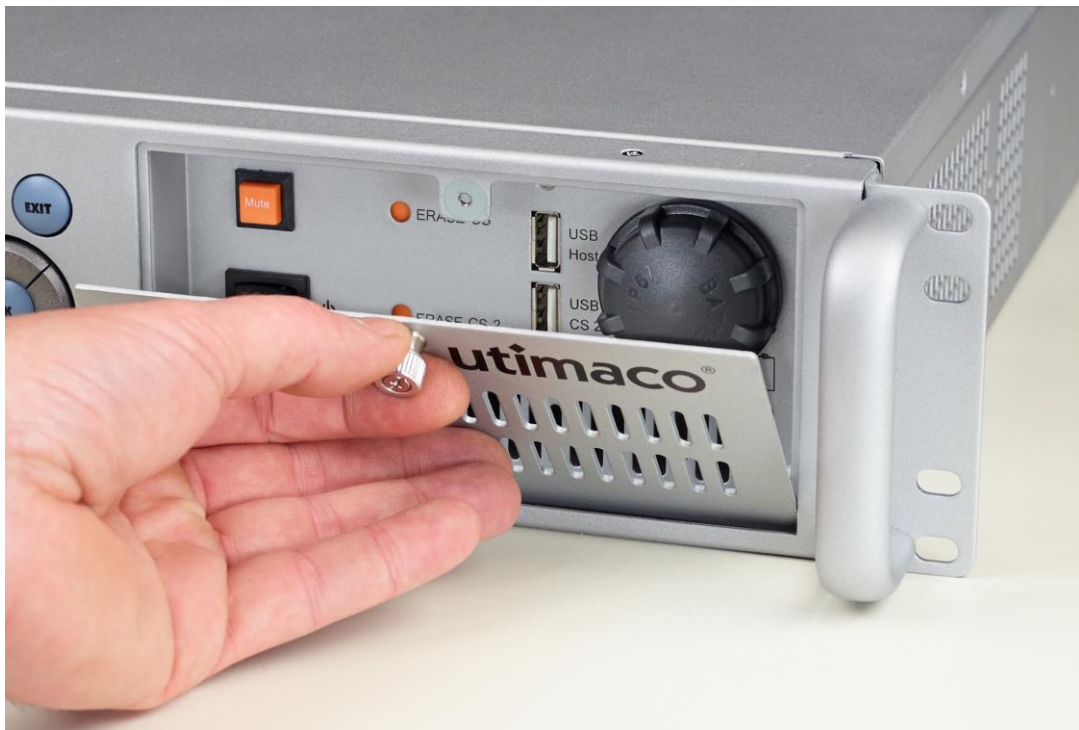
Figure 13: Opening the front door of the CryptoServer LAN V4
