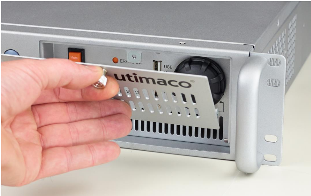
Figure 14: Removing the front door of the CryptoServer LAN V4
