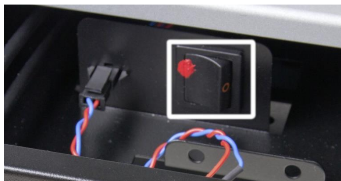
Figure 12: Rocker switch for performing External Erase on a CryptoServer LAN V3
