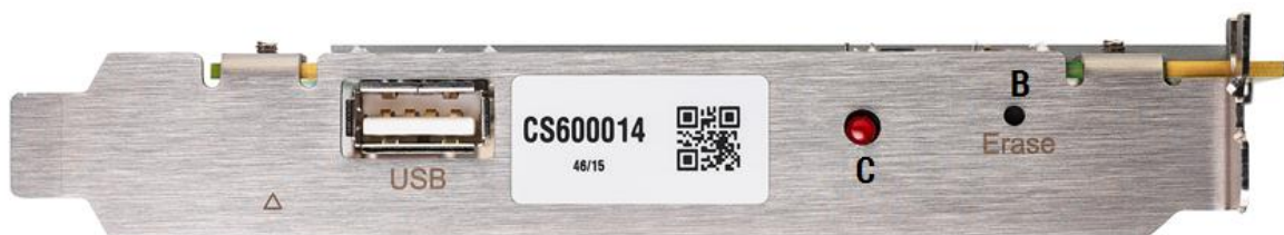
Figure 12: Performing External Erase on a CryptoServer Se-Series Gen2 plug-in card
