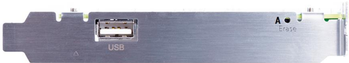
Figure 11: Performing External Erase on a CryptoServer CSe-Series plug-in card
