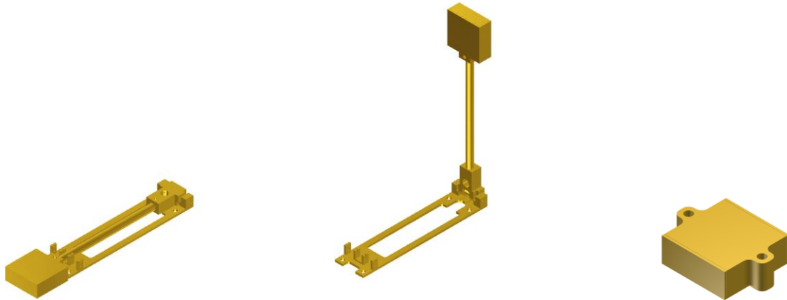
Figure 7 - Stowed, deployed and redundant magnetometer
