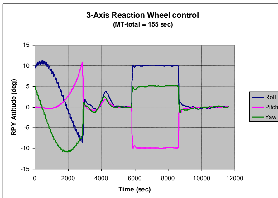
Figure 16: Reaction wheel control performance in Control Stage 3 without CubeStar
