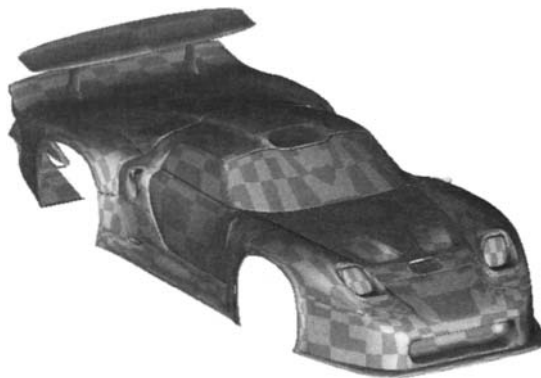
Figure 21.15 Surface splines: an example. (Courtesy J. Peters.)
