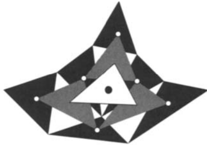
Figure 17.2 The “triangular” de Casteljau algorithm: a point is constructed by repeated linear interpolation.
