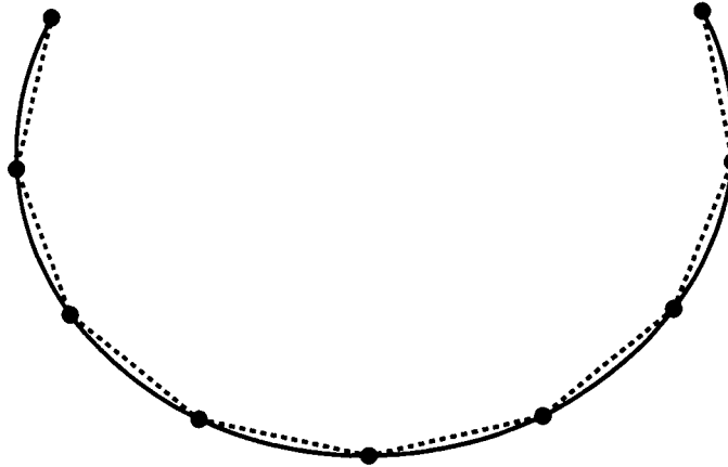
Figure 9.10 Bessel end condition spline.
