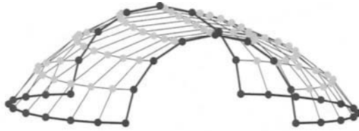
Figure 15.3 Coons patches: an example for n = 11 and m = 9 .
